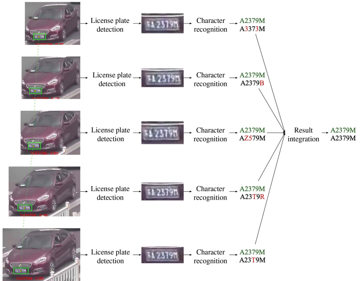
Figure 1: Framework of the LPR System Based on Vehicle Tracking and Result Integration.
