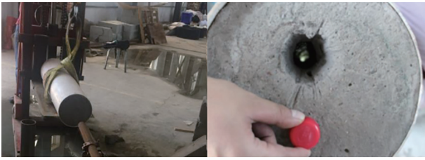
图 12 旋转多孔喷嘴破岩实验(人造砂岩) Fig. 12 Rock breaking experiment with rotating porous nozzle (artificial sandstone)
