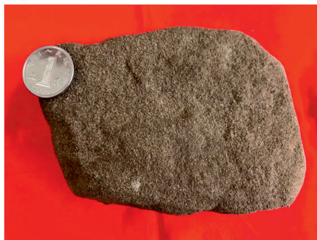
NP1-5, 2717.40 m, Ed 1 , oil-bearing sandstone sample.
