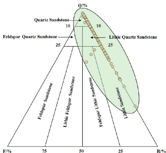
**Figure 4.** Characteristics of tight sandstone reservoir composition of Benxi Formation in Ordos Basin (280 samples). Q represents quartz content. F represents feldspar content. R represents lithic content. The data are almost distributed in the area of quartz sandstone, lithic quartz sandstone, and lithic sandstone. Only two samples are feldspar lithic sandstone. There is no feldspar quartz sandstone, feldspar sandstone, or lithic feldspar sandstone in the study area.
