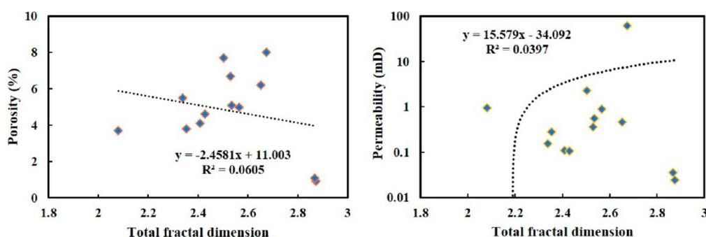
Figure 12. Relationship between total fractal dimension and porosity and permeability.
