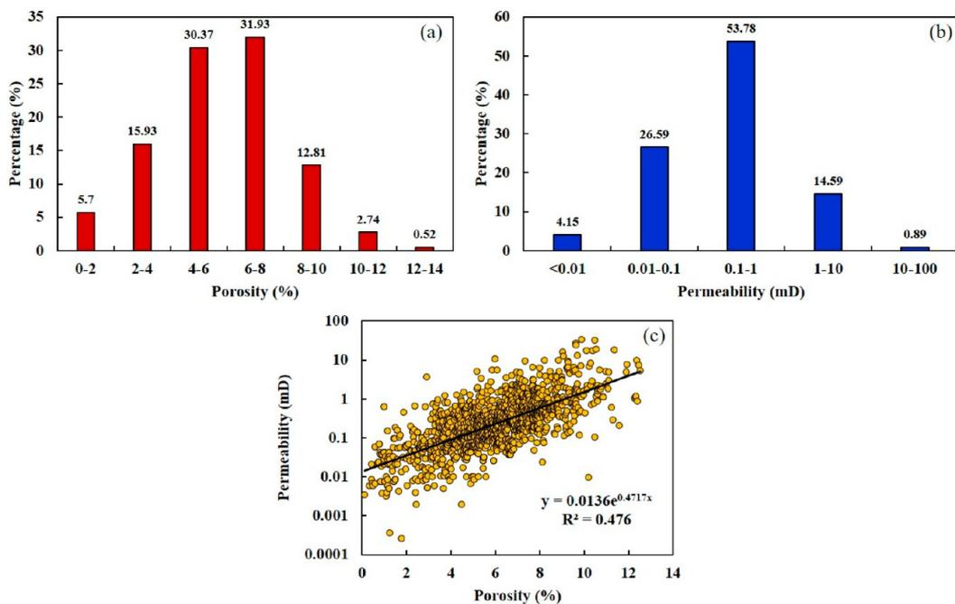
Figure 5. Porosity and permeability histogram and porosity and permeability scatter plot.
