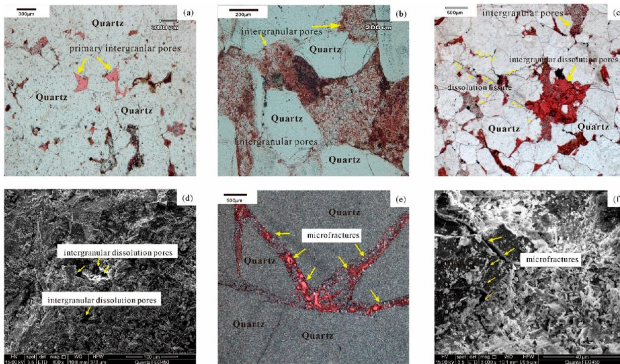
Figure 6. Thin section and scanning electron microscope image of tight sandstone in coal measure of Benxi Formation: (a) primary intergranular pores between quartz particles, (b) intergranular pores formed by clay minerals, (c) dissolution pores of harborlike, (d) intergranular dissolution pores between grains, (4) well-developed microfractures, and (f) microfractures between brittle minerals.
