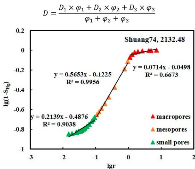
**Figure 11.** Fractal analysis for heterogeneity interpretation of pore network, taking sample Shuang 74 as an example.
