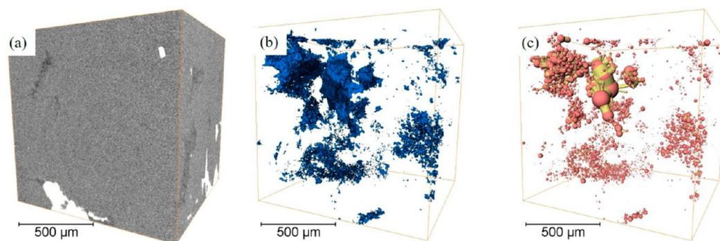
**Figure 10.** Three-dimensional CT images of Shan 336. (a) Three-dimensional CT image of the sample. (b) Three-dimensional pore structure model. (c) Three-dimensional pore throat network model. The pink balls in the pore throat network model represent pores, and the yellow rods represent throats.
