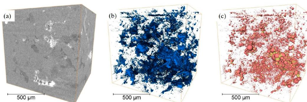
**Figure 9.** Three-dimensional CT images of Qi17. (a) Three-dimensional CT image of the sample. (b) Three-dimensional pore structure model. (c) Three-dimensional pore throat network model. The pink balls in the pore throat network model represent pores, and the yellow rods represent throats.
