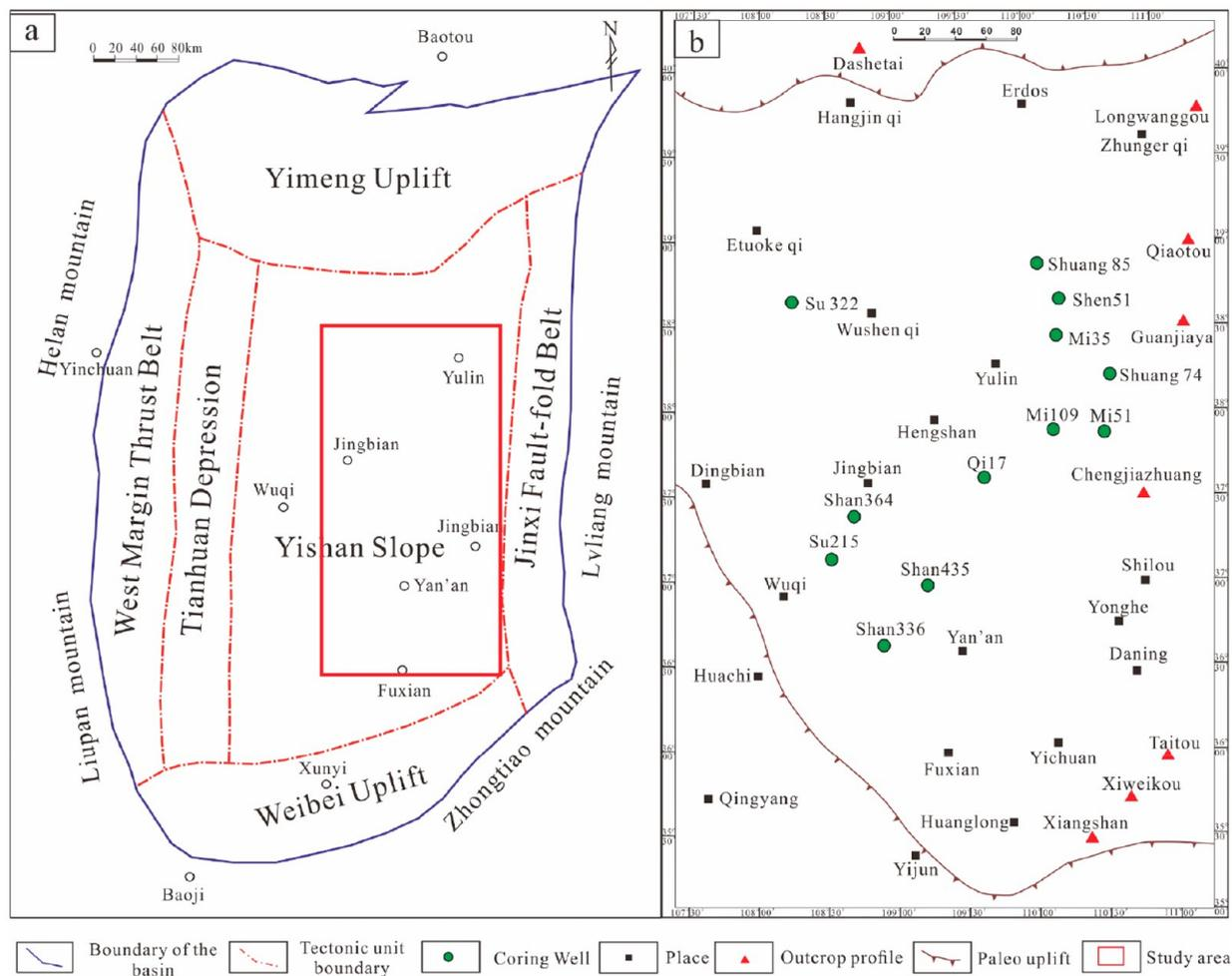
**Figure 1.** (a) Structural units of the Ordos Basin. (b) The location of Coring well.
