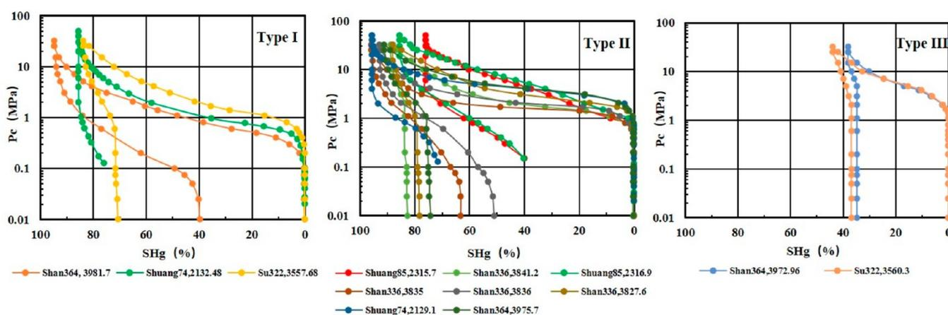
**Figure 7.** Different types of mercury injection curve.
