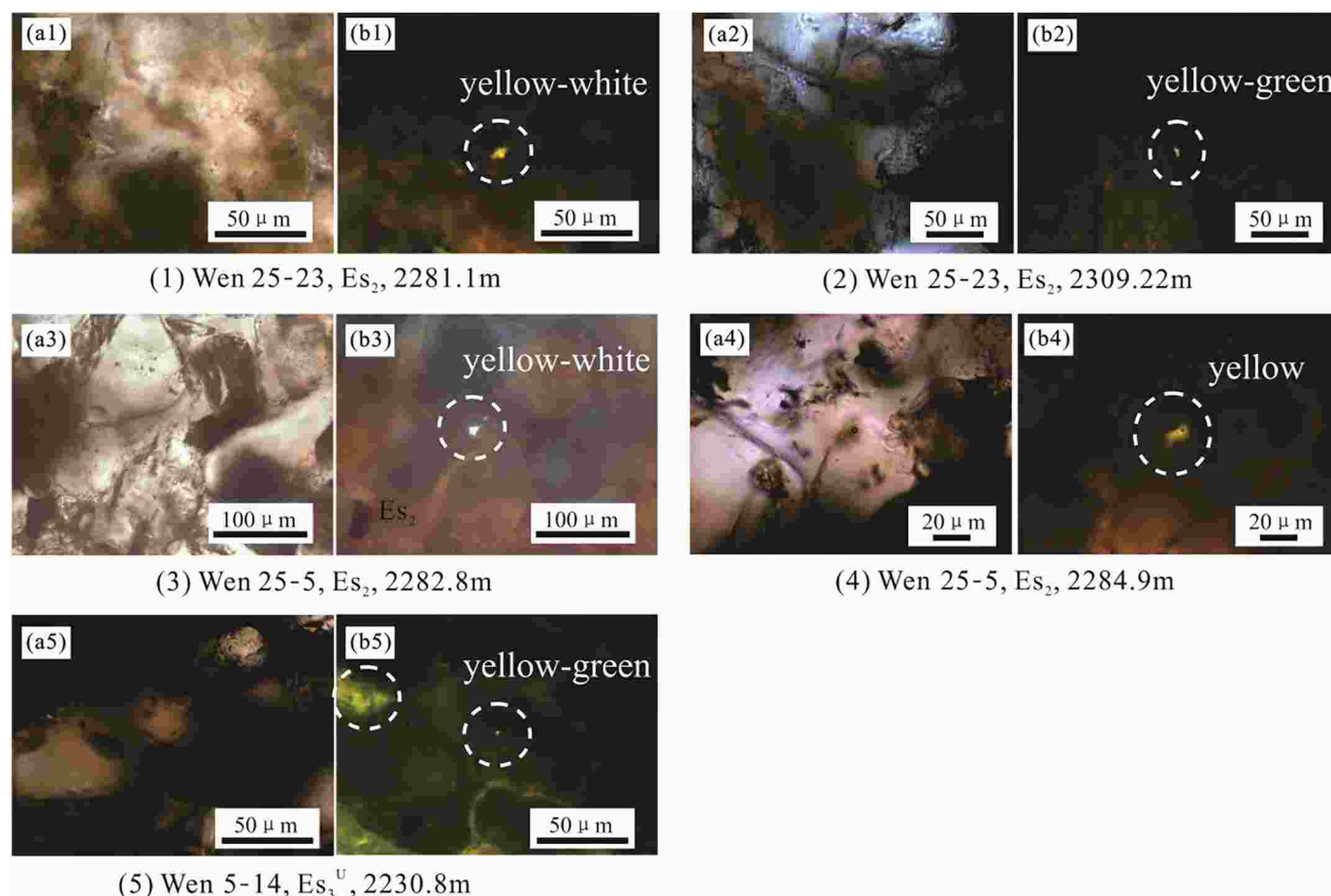
Fig. 8. Petroleum fluid inclusion images of Es_2 and Es_3^U sandstones in structural high position in DCHA of eastern Wenliu area, Dongpu Depression.
