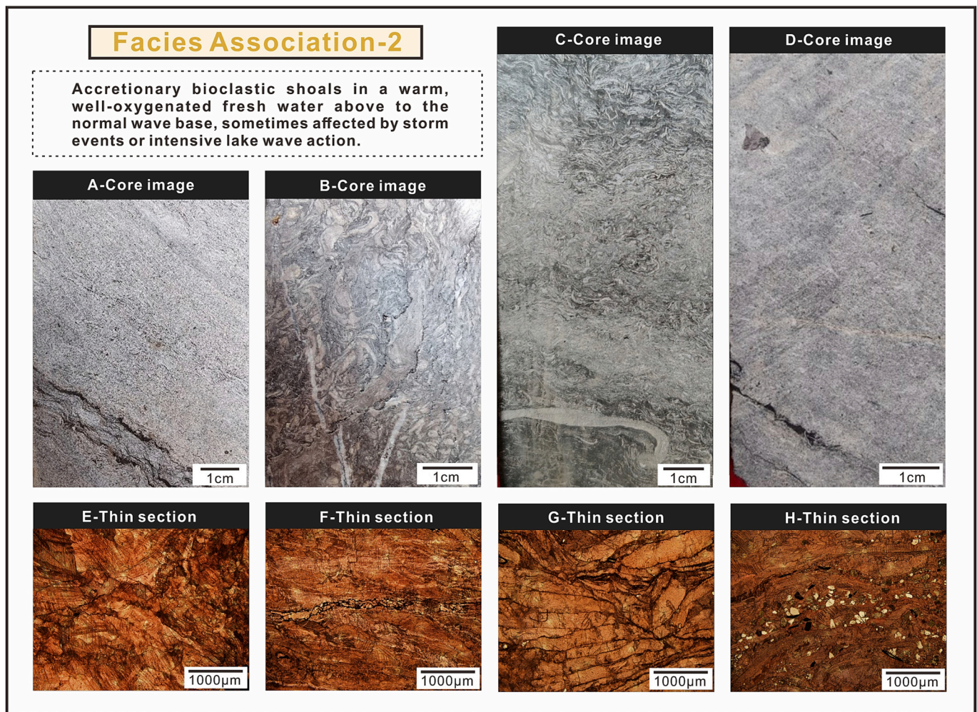
Fig. 4. Overview and examples of key features for FA2. (A) Fossiliferous carbonate with parallel-to-wavy bedding, primarily consisting of bivalve and ostracod shell fragments. Well X1, 3154.20 m; (B) Fossiliferous carbonate composed of randomly scattered bivalve and ostracod shell fragments. Well X1, 3106.75 m; (C) Fossiliferous carbonate with chaotic beddings. Well X1, 3160.00 m; (D) Calcified bioclasts are generally intact to broken. Well X1, 3192.80 m; (E) Carbonate minerals are almost all dyed red by stain. Elongate bioclastic occurs in randomly scattered distribution. Well X1, 3128.57 m, PPL; (F) Carbonate minerals are almost all dyed red by stain. Elongate bioclastic occurs in the slight imbrication distribution. Well X1, 3155.19 m, PPL; (G) Carbonate minerals are almost all dyed red by stain. Elongate bioclastic occurs in the imbrication distribution. Well X1, 3160.12 m, PPL; (H) Silty quartz and feldspar grains oriented in the elongate bioclastic. Well X1, 3191.94 m, PPL. PPL: plane-polarised light. (For interpretation of the references to colour in this figure legend, the reader is referred to the web version of this article.)
