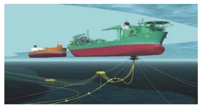
A: FPSO (floating production, storage and offloading)
