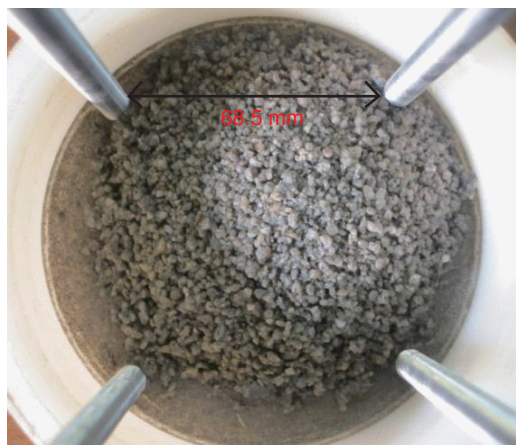
Fig. 8 Produced sand in the sand trap for sample G
