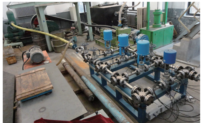
Fig. 5 The parallel choke for measuring pressure characteristics
