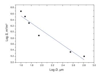
Fig. 3 The relationship of the specific surface area of anorthite and its grain diameter
