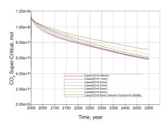
**Fig. 4** Quantity of supercritical CO<sub>2</sub> with time for anorthite and calcite with different reactive surface areas
