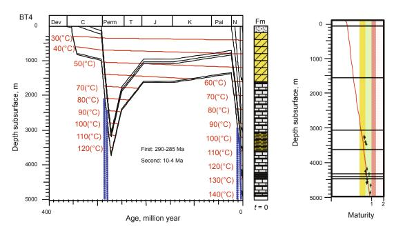
Fig. 8 Burial and thermal history of D<sub>3</sub>d in well BT4 in the Bashituo Oilfield
