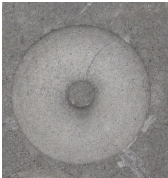
Fig. 7 The rock sample cut by the micro PDC bit (sample 1#)
