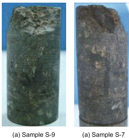
Fig. 10 The end of core flaked off after immersion
