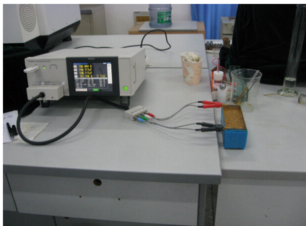
Fig. 8 A plastic container with copper plate and sand saturated with NaCl solution, the dimension is length × width × height = 17 cm × 5.0 cm × 4.7 cm
