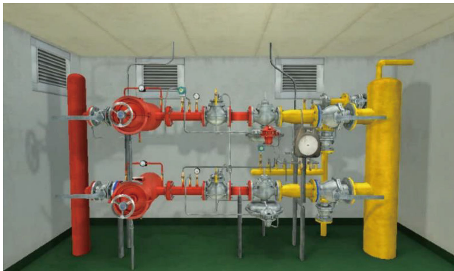
Fig. 4 3D image of a pressure-regulating station
