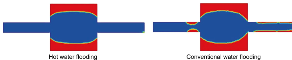
Fig. 18 Difference in residual oil and water distribution between conventional and hot water flooding after water broke through (Lv and Wang 2015)
