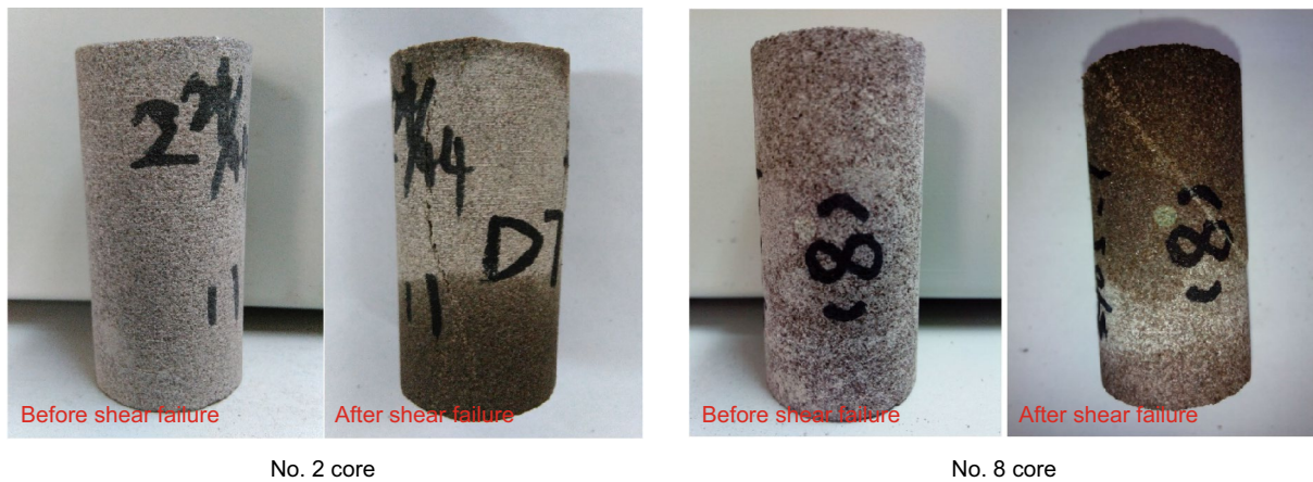
Fig. 1 Core samples before and after shear failure
