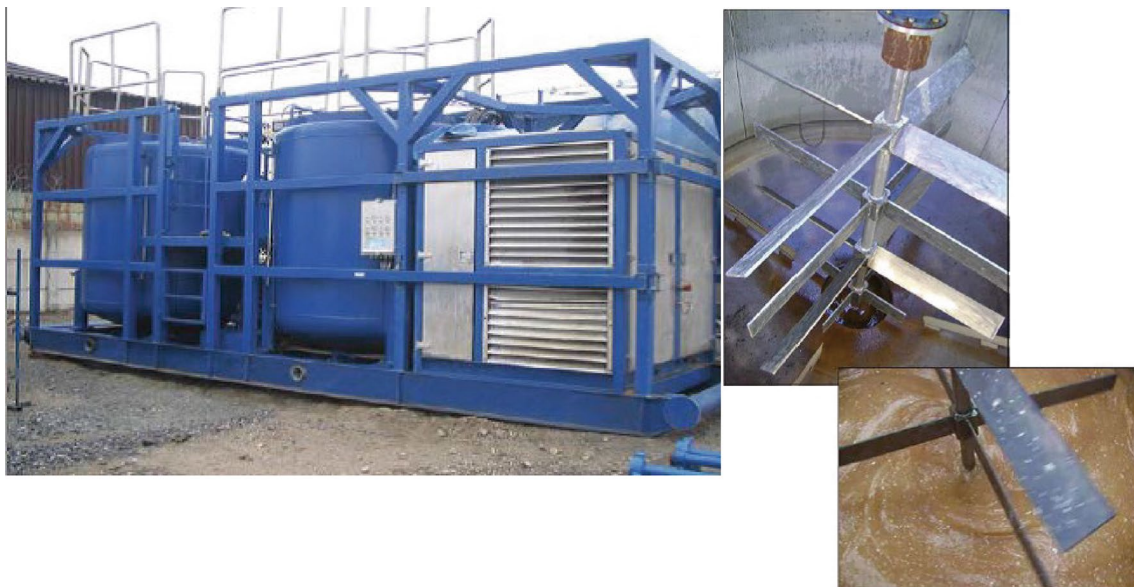
Fig. 9 Batch mixing of the degradable diverting acid system (Asiri et al. 2013)
