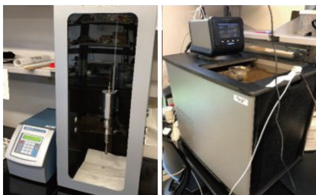
Fig. 3 Q-Sonica Q500 ultrasonicator in a sound enclosure (left) and PolyScience temperature-controlled bath (right)
