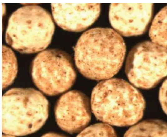
Fig. 5 Picture showing the sphericity of ULW-3 (Jardim Neto et al. 2012b)
