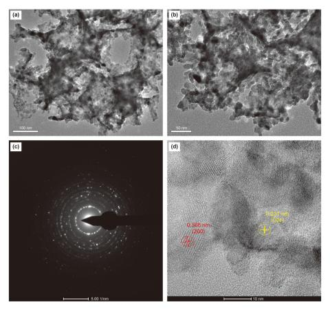
Fig. 5. a, b TEM images, c SAED image and d HR-TEM image of 3DOM W-TiO<sub>2</sub>-20.
