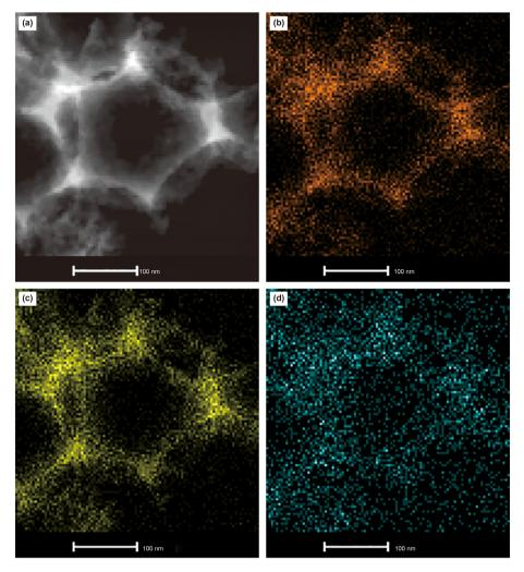
Fig. 6. TEM-mapping images of 3DOM W-TiO<sub>2</sub>-20.
