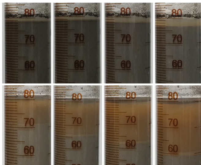
Fig. 1. Experiment of drilling fluid carrying rock cuttings. (a) 4% bentonite + 10% NaCl + barite ( \rho = 2.0 \text{ g/cm}^{-3} ) after ageing at 180 °C for 16 h; (b) 4% bentonite + 10% NaCl + 0.05% carbon nanotube + barite ( \rho = 2.0 \text{ g/cm}^{-3} ) after ageing at 180 °C for 16 h.
