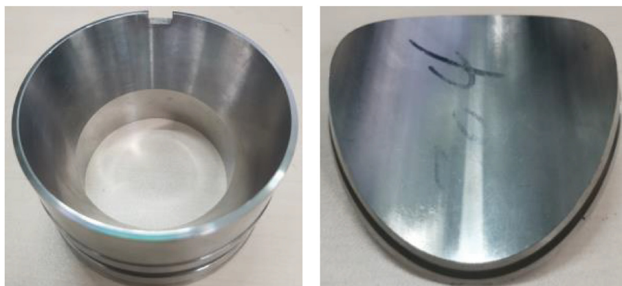
Fig. 16. Key components of the pressure controller.
