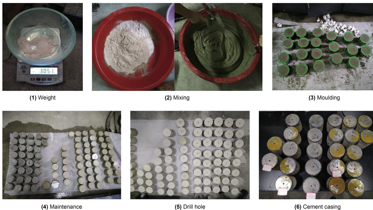
Fig. 2. The schematic procedure for preparing artificial specimens.
