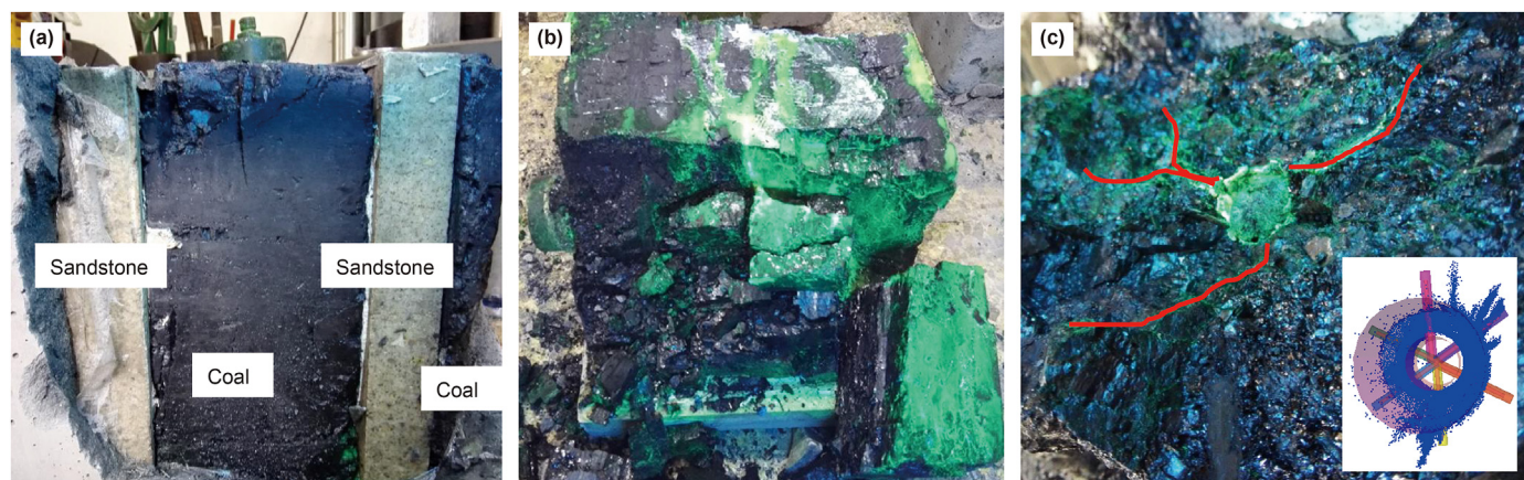
Fig. 19. Laboratory true-triaxial experiment to simulate Scheme 3. (a) The specimen before fracturing; (b) and (c) Fracture morphology after fracturing.
