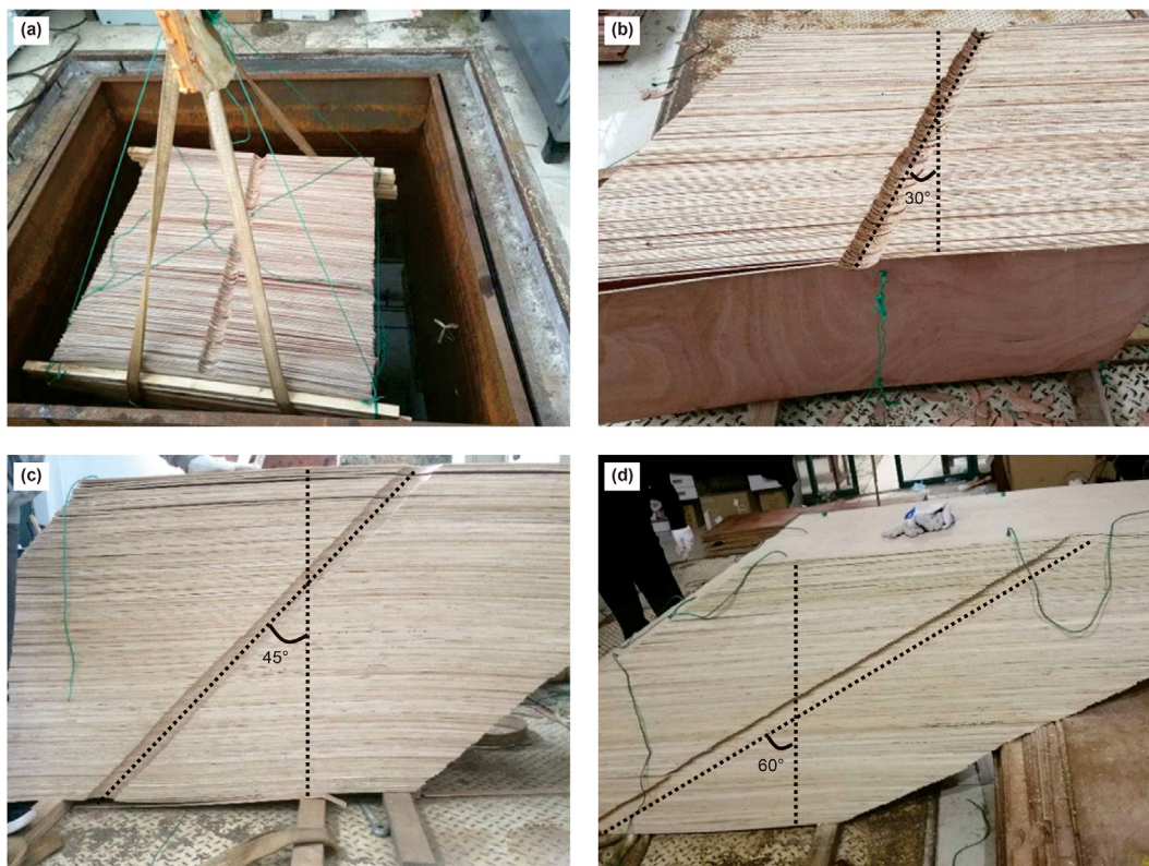
Fig. 8. Formation models with different dipping angles: (a) \theta = 0^\circ ; (b) \theta = 30^\circ ; (c) \theta = 45^\circ and (d) \theta = 60^\circ .
