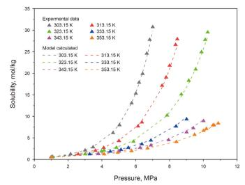
Fig. 12. Comparison of the experimental values of  $CO_2$  solubility in n-dodecane with those calculated from a model.
