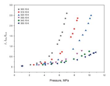
Fig. 9. Raman peak intensity ratios of the CO  $_2$  + n-dodecane system at 303.15–353.15 K and 1.00–11.00 MPa.
