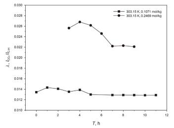
Fig. 4. The change in the  $CO_2$  + n-dodecane Raman peak intensity ratio with time under different  $CO_2$  concentrations at 303.15 K.
