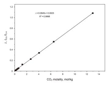
**Fig. 8.** The relationship between  $CO_2$  molality and the Raman peak intensity ratio between the upper band of  $CO_2$  Fermi diad and n-dodecane derived from spectra collected from homogeneous  $CO_2/n$ -dodecane solutions.
