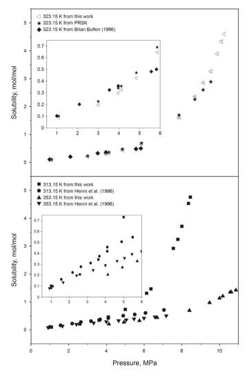
**Fig. 11.** Comparison of the  $CO_2$  solubilities in n-dodecane obtained in this study with those reported previously.
