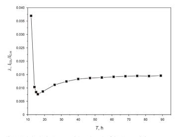
Fig. 3. Variation in the Raman peak intensity ratio of the CO<sub>2</sub> + n-dodecane system with time (T = 293.15 K, P = 6.67 MPa,  $x_{CO_2} = 0.1071$  mol/kg).
