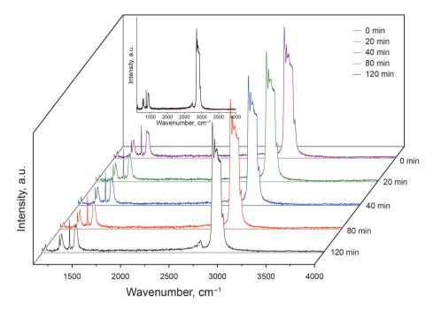
Fig. 7. Raman spectra of the CO<sub>2</sub> + n-dodecane system at 333.15 K and 5.55 MPa from 0 to 120 min after phase equilibrium was reached.
