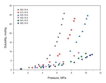
Fig. 10. Solubility of  $CO_2$  in *n*-dodecane at 303.15–353.15 K and 1.00–11.00 MPa.
