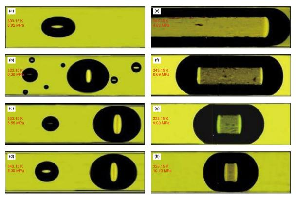
Fig. 5. Changes in the CO<sub>2</sub>-saturated solution during heating and depressurization (a)  $\rightarrow$  (d), and cooling and pressurization (e)  $\rightarrow$  (h) in a FSC.
