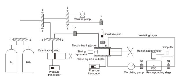
Fig. 2. Schematic diagram of the CO<sub>2</sub> + n-dodecane solubility measurement system. 1 to 13 are high-pressure valves. FSC = fused silica capillary.
