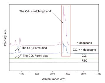
Fig. 1. Raman spectra of CO<sub>2</sub>, n-dodecane, and fused silica capillary (FSC).
