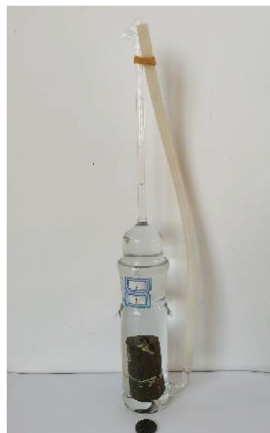
Fig. 1. Imbibition cell with the accuracy of 0.01 mL.
