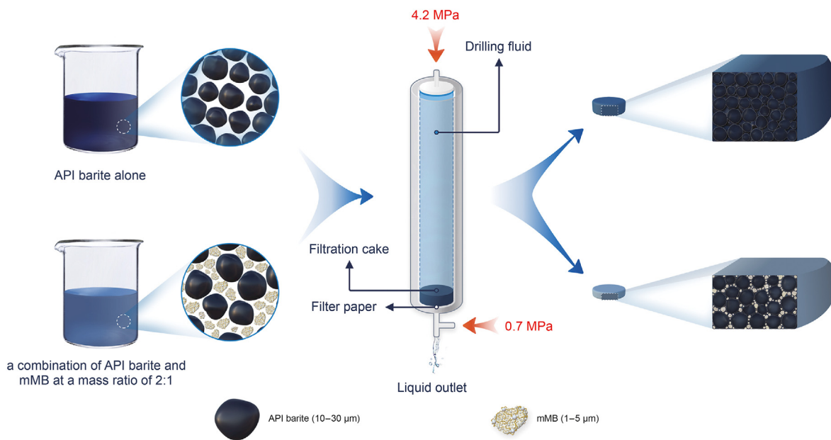
Fig. 8. Mechanism of WBDFs weighted with a combination of API barite/mMB in regulating rheological properties and filtration performance.
