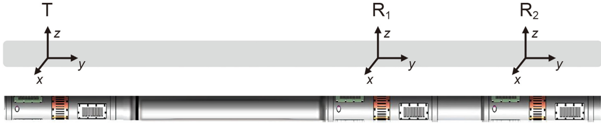
Fig. 1. Three-component transceiver antenna structure of the LWD look-ahead resistivity instrument, where T represents the transmitting antenna, and R_1 and R_2 represent the first and second receiving antenna, respectively.
