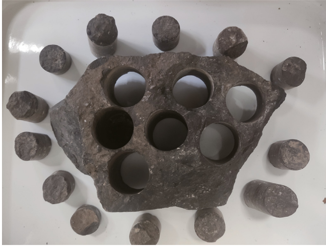
Fig. 3. Pre-prepared cylindrical core samples.
