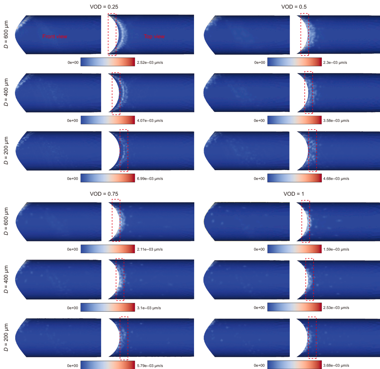
Fig. 19. Contour of downstream erosion rate distribution.
