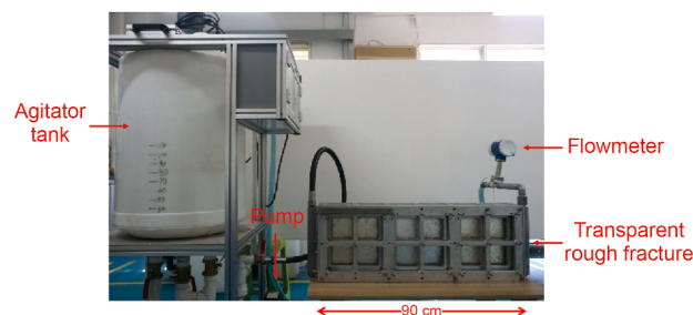
Fig. 3. Visualized rough fracture model for evaluating the proppant-carrying ability of the fracturing fluid.
