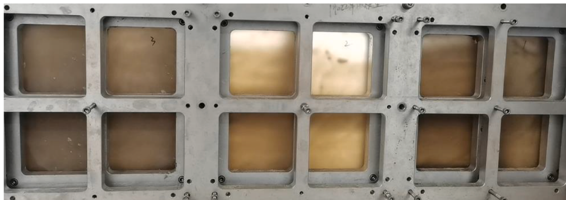
Fig. 8. Slurry flows in the transparent rough fracture model without settling (0.2% viscous slickwater, 20% sands, and an intra-fracture velocity of 12.5 m/min).
