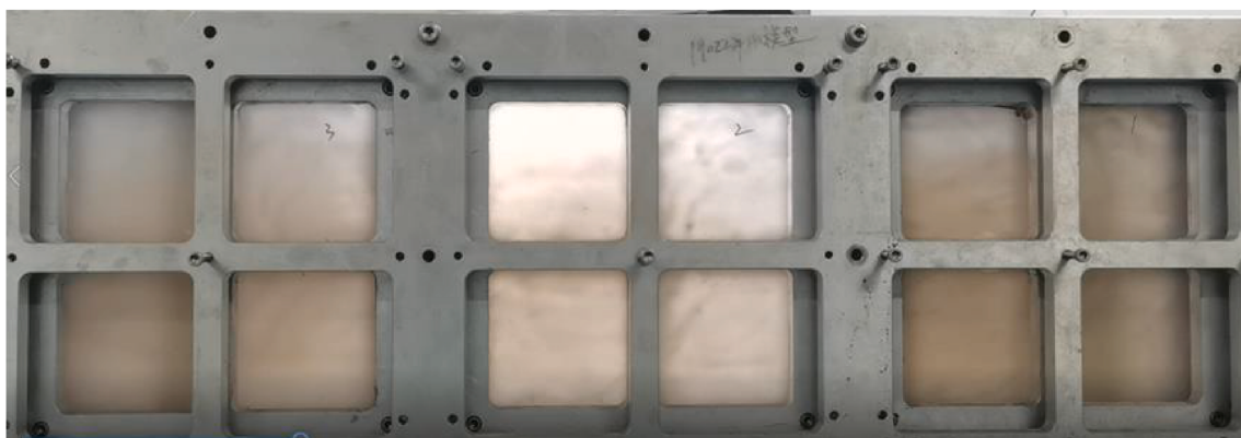
Fig. 15. Slurry flows in the transparent rough fracture model with settling (0.2% viscous slickwater in the deionized water, 10% sands, and an intra-fracture velocity of 8 m/min).
