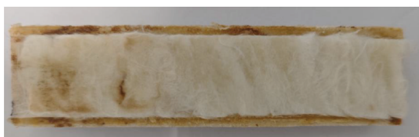
Fig. 5. Distribution of fibers within the fracture.
