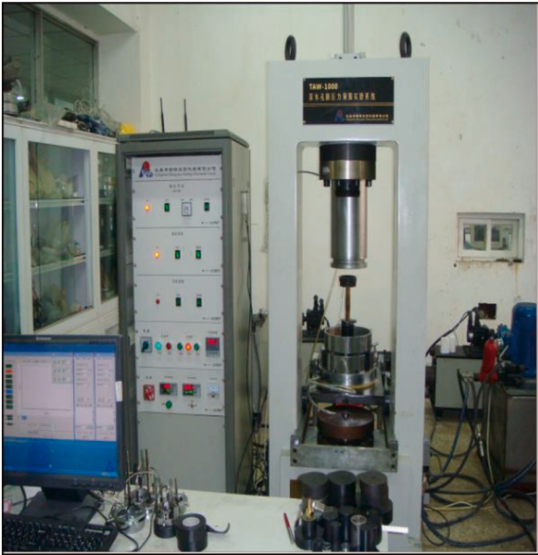
Fig. 7. Device diagram of the TAW-1000 Deepwater Pore Pressure Servo Test System.
