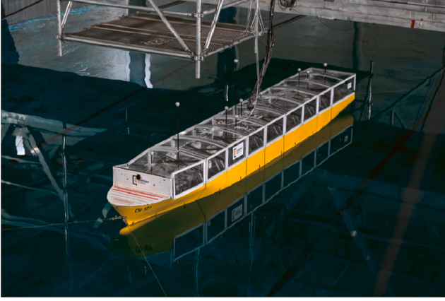
Fig. 8. Ship model and experimental setup (adopted from Dermatis et al. (2025)).
