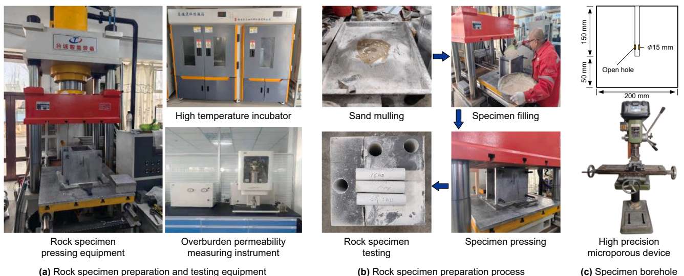
Fig. 2. Fabrication process of multilayer heterogeneous rock specimens.
