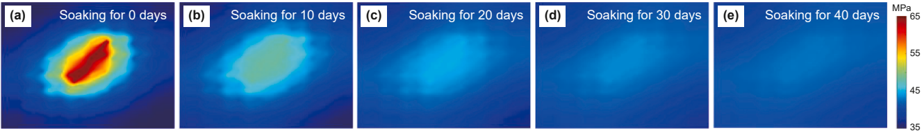
Fig. 15. Rock damage zones formed by fracturing-flooding water injection under different natural fracture densities. (a) Soaking for 0 days. (b) Soaking for 10 days. (c) Soaking for 20 days. (d) Soaking for 30 days. (e) Soaking for 40 days.
