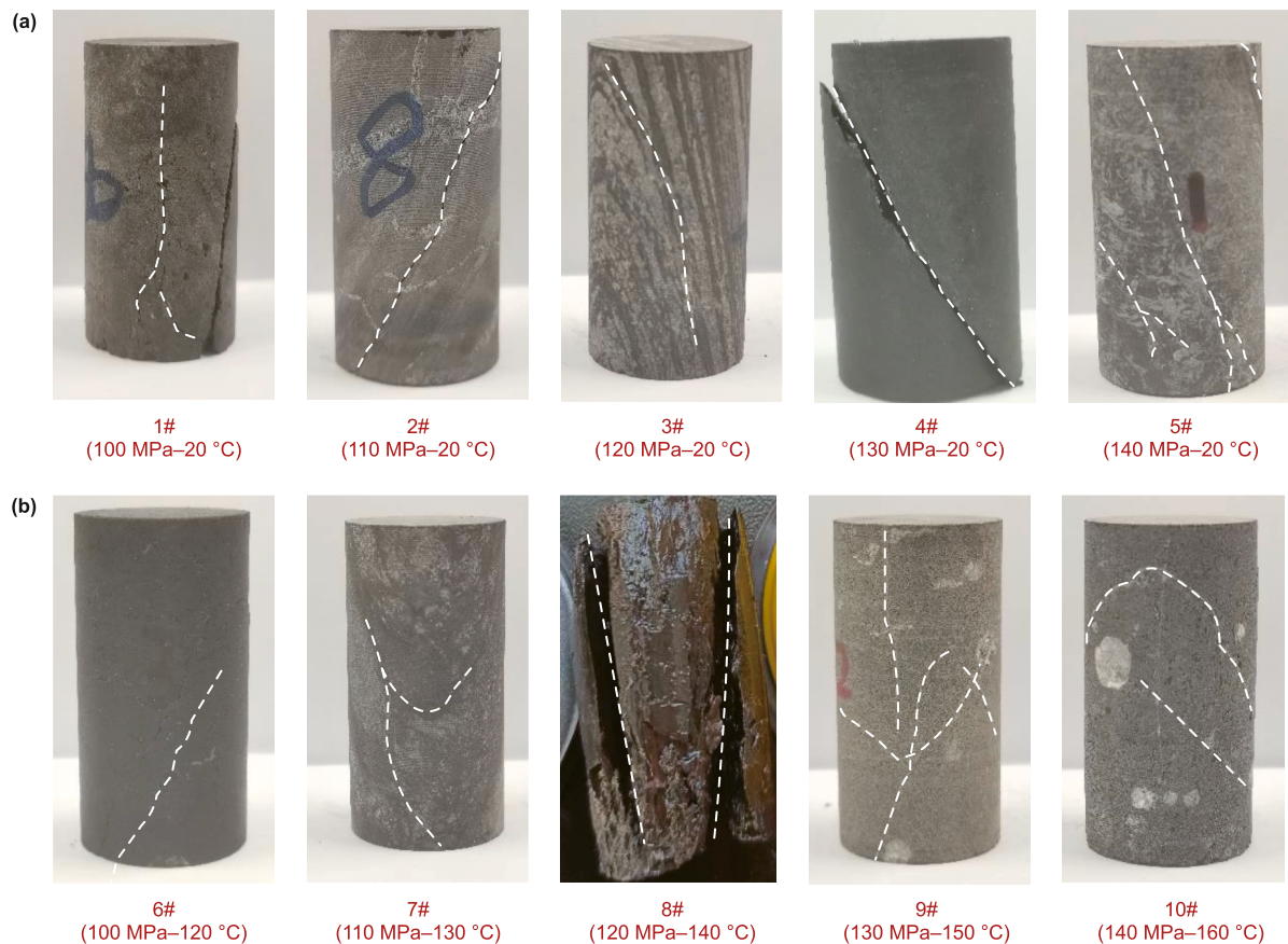
Fig. 4. Failure modes of ultra-deep rocks under different conditions. (a) HPAT conditions; (b) HPHT conditions.
