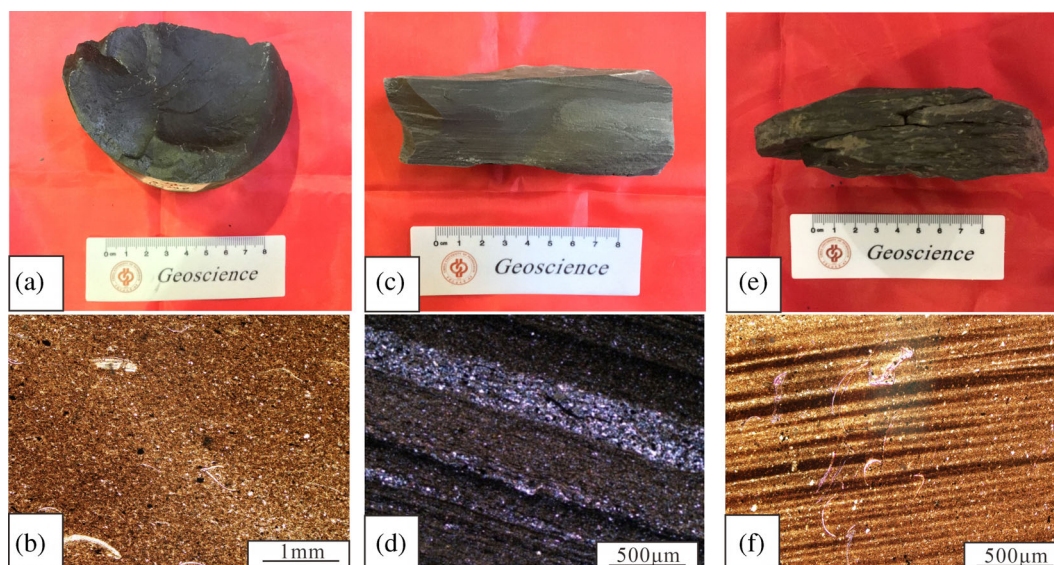
FIGURE 5 Major sedimentary structure types of the shale in plane-polarized light. a and b: laminated structure (<1 mm); c and d: bedded structure (1 cm >> 1 mm); e and f: massive structure
