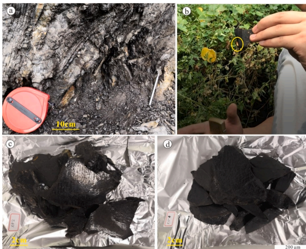
Fig. 2. Generalized features of black shales of the Xiamaling Formation. (a) the outcrop of black shales of Xiamaling Formation in the Xiahuayuan area (XHY), Hebei province. A pickaxe was used to remove vegetation and oxidized layers on the surface, then exposing fresh rocks; (b) ignition of the black shales; (c-d) the outcrop samples of black shales collected from XHY section depicting organic-rich layers.
