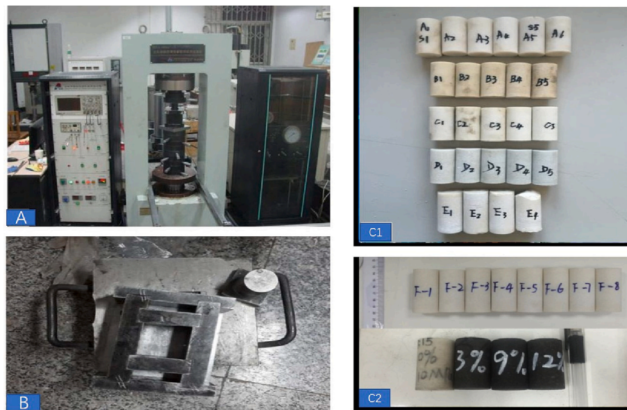
Fig. 6. Physical simulation experiment equipment for artificial core preparation and obtained artificial core samples. A- Artificial core compactor; B- Artificial core mold; C- Artificial core photographs A-E series (C1) and F-G series (C2).
