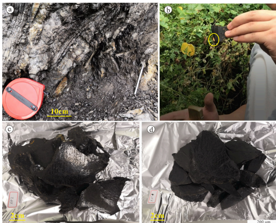
Fig. 2. Overview of the characteristics of black shales from the Xiamaling Formation. (a) The outcrop of the Xiamaling Formation black shales in the Xiahuayuan area (XHY), Hebei province. The vegetation and oxidized surface layers were removed using a pickaxe, exposing fresh rock surfaces; (b) Ignition of the black shales; (c-d) The outcrop samples of black shales from the XHY section (modified from [22]).
