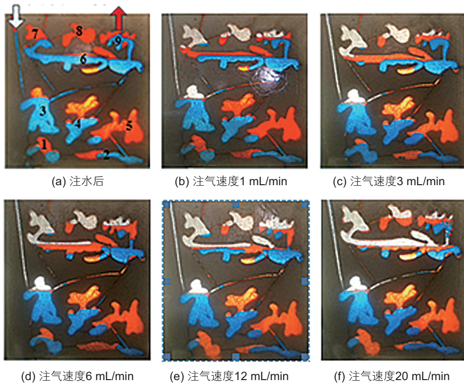
图5 不同注气速度油水分布对比 Fig. 5 Oil/water distribution comparison with N 2 injection at different speeds
