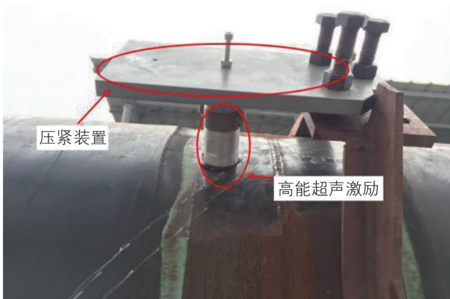
图 13 管道焊接残余应力调控现场 Fig. 13 Regulation site picture of pipeline welding residual stress
