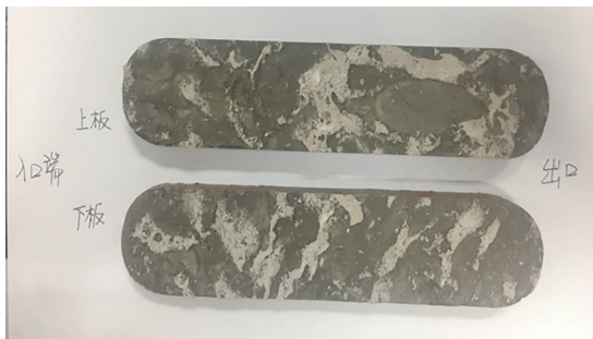
图5 酸蚀16 min后的导流板 Fig. 5 The guide plate after 16 min of acid etching
