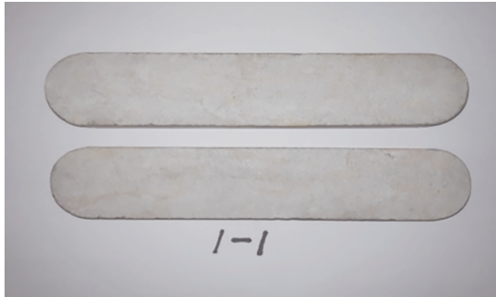
图4 酸蚀岩板 Fig. 4 Samples before acid etching
