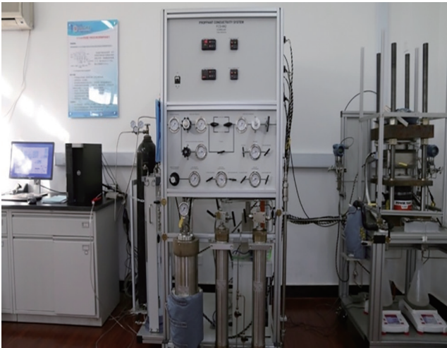
图 11 FCS-842 导流仪 Fig. 11 FCS-842 Hydraulic fracture conductivity test system
