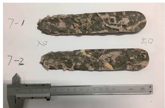
图7 酸蚀56 min后的导流板 Fig. 7 The guide plate after 56 min of acid etching
