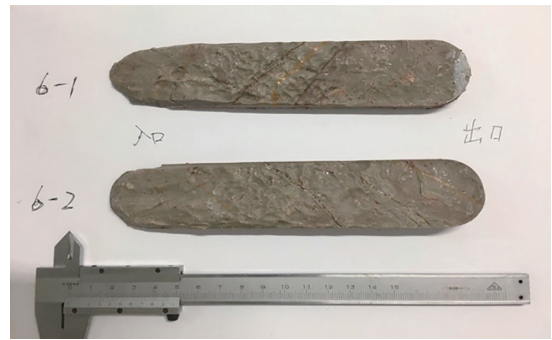
图6 酸蚀46 min后的导流板 Fig. 6 The guide plate after 46 min of acid etching
