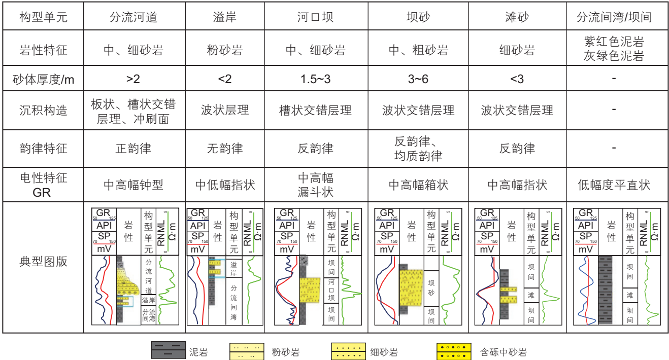
图 6 东营凹陷胜二区不同类型构型单元的测井解释模板 Fig. 6 Well logging interpretation templates for different types of architectural units in the 2nd Block of Shengtuo Oilfield, Dongying Sag
