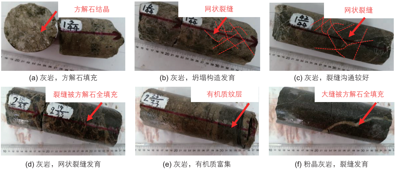
图 3 W 井岩心裂缝发育情况图 Fig. 3 Core fracture development of well W
