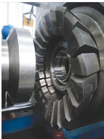
图 7 干涉的卡爪 Fig. 7 Claws in the interference state
