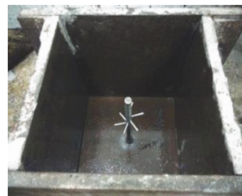
图7 井筒及模具组合 Fig. 7 Assembly of wellbore and cast model
